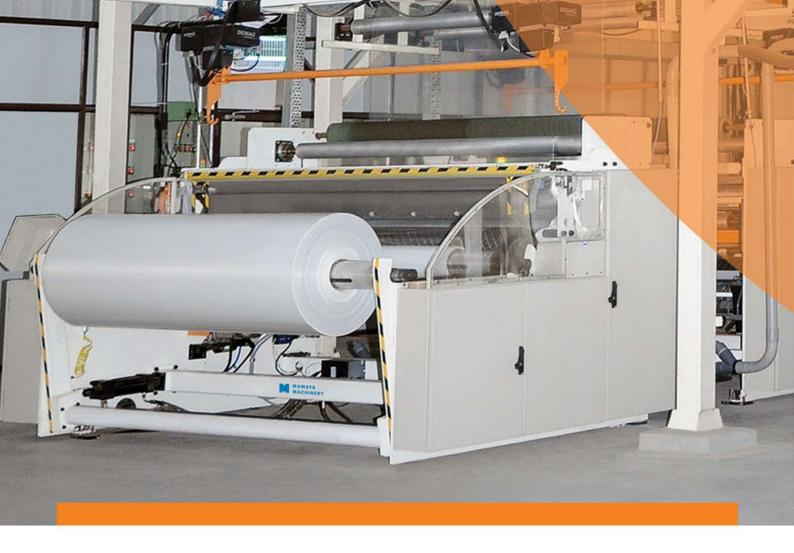
The right selection of width of the post extrusion equipment of the Blown Film Line will take care of matching widths of converting equipment like Printing, Lamination, Slitting, Bagging / Pouching machines etc.
